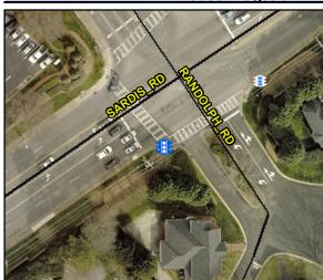
Possible Solutions: Replace Signal Push Button With APS Button on New Post. Remove & Relocate Sign. Provide Push **Button Extension.**
