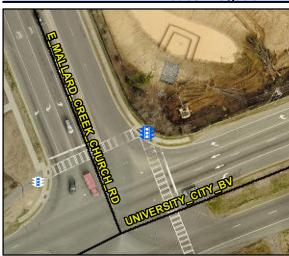
Possible Solutions: Replace Signal Push Button With APS Button on New Post. Remove & Relocate Sign.
