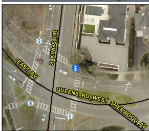
Possible Solutions: Replace Signal Push Button With APS Button on New Post. Remove & Relocate Sign. Provide PAR As Indicated. Provide Clear Space.
