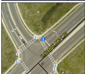
Possible Solutions: Provide Push Button Extension. Remove and Replace Clear Space.
