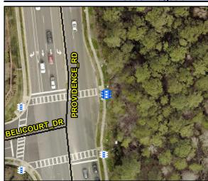
Possible Solutions: Replace Signal Push Button With APS Button on New Post. Remove & Relocate Sign. Surveyor Notes: N/A PROW/ADA: TMUTCD 4e.08. R404.2 Total Cost:
