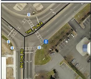
Possible Solutions: Remove & Replace Crossing Striping. Adjust Signal Button Height. Provide Push Button Extension. Remove and Replace Clear Space.
