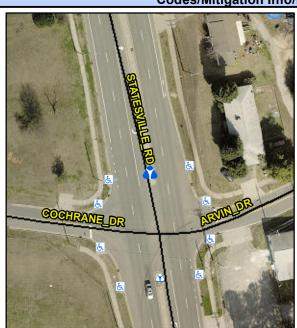
Grind Gutter Lip. Remove & Replace Gutter.
