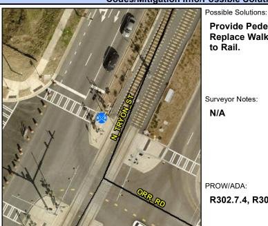
**Provide Pedestrian Gate. Remove & Replace Walking Surface Adjacent** to Rail.
