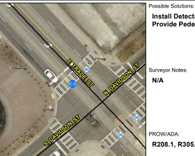
Install Detectable Warning System. Provide Pedestrian Gate.
