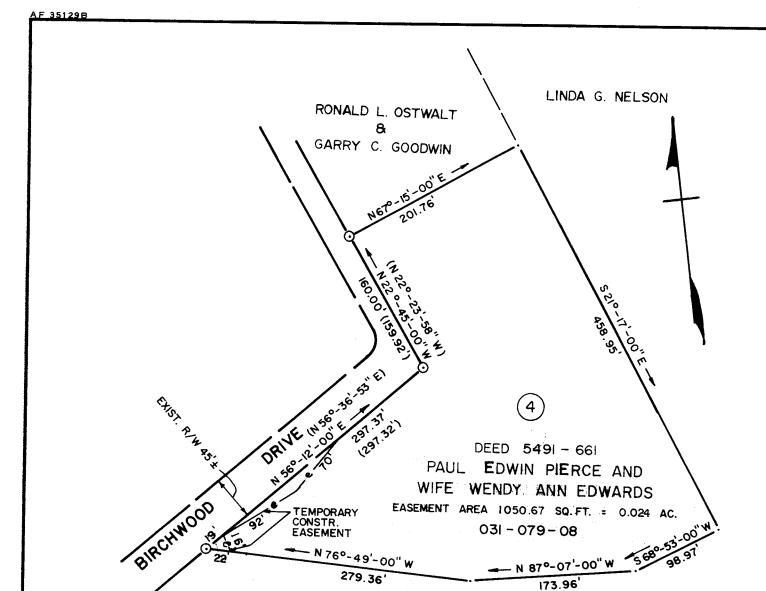
Note: Property corners shown circled were located by actual survey. Bearings and distances are based on:
