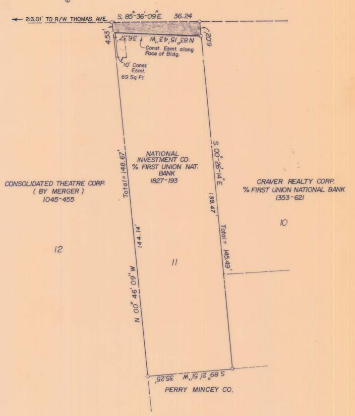
WOTE: PROPERTY CORNERS NOTED WERE LOCATED BY ACTUAL SURVEY BEARINGS ARE BASED ON DEED BOOK 2747 PAGE 477. THIS MAP WAS PREPARED FOR THE PURPOSE OF RIGHT OF WAY OR EASEMENT ACQUISIT-ION ONLY, AND IS NOT INTENDED TO BE A BOUNDARY SURVEY OF THE PROPERTY SHOWN
