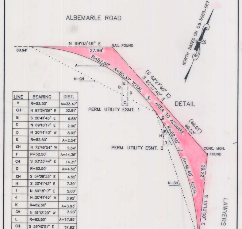
TOTAL AREA ( BY DEED ) 29,453 S.F.=0.6762 AC. AREA TO ACQUIRE 975 S.F.=0.0224 AC. PERM. UTILITY ESMT. 1 18 S.F.=0.0004 AC. PERM. UTILITY ESMT. 2 11 S.F.=0.0003 AC. AREA REMAINING 28,449 S.F.=0.6537 AC. TEMP. CONSTR. ESMT.
