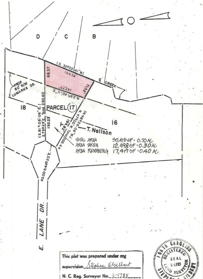
NOTE: Property corners shown circled were located by actual survey. Bearings are based on N.C. GRID
