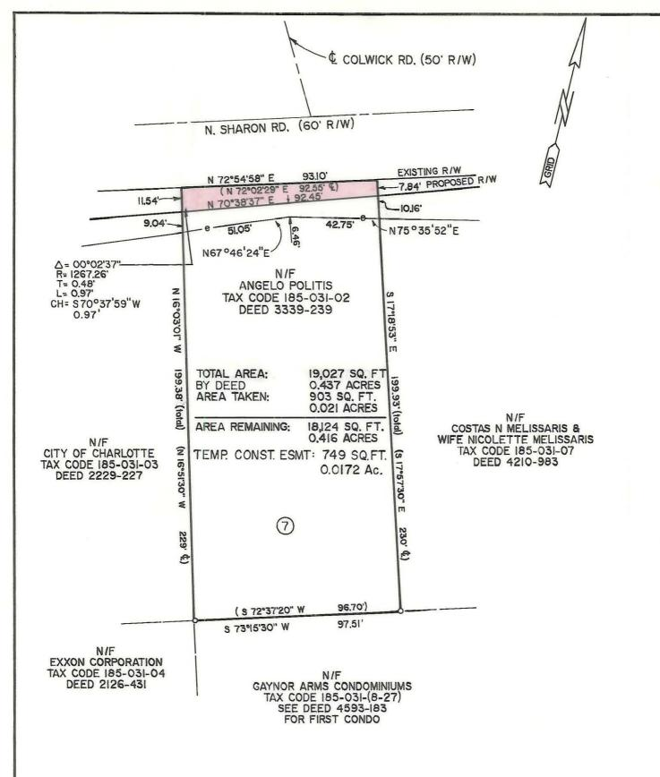
PROPERTY CORNERS SHOWN CIRCLED WERE LOCATED BY ACTUAL SURVEY. BEARINGS AND DISTANCES SHOWN IN PARENTHESIS ARE BASED ON DEED INFORMATION, BEARINGS ARE BASED ON THE N.C. STATE GRID SYSTEM.
