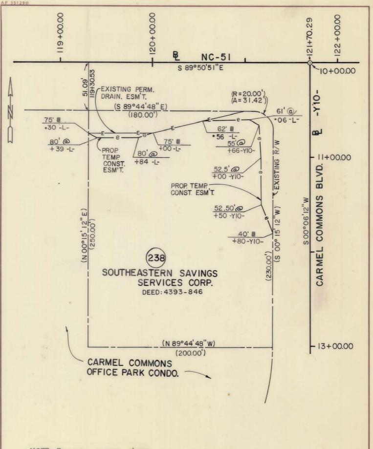
NOTE: Property corners shown circled were located by actual survey. Bearings and distances shown in parenthesis are based on deed information. Bearings are based on
