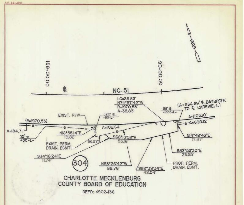
NOTE: Property corners shown circled were located by actual Bearings and distances shown in parenthesis are based on deed information. Bearings are based on
