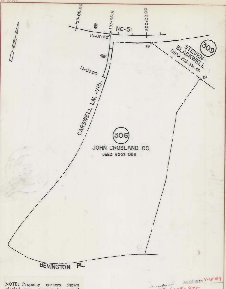
circled were located by actual Bearings and distances survey. shown in parenthesis are based on deed information. Bearings are based on
