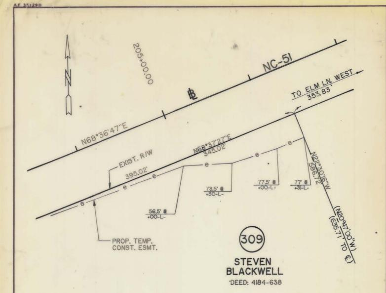
NOTE: Property corners shown circled were located by actual survey. Bearings and distances shown in parenthesis are based on deed information. Bearings are based on
