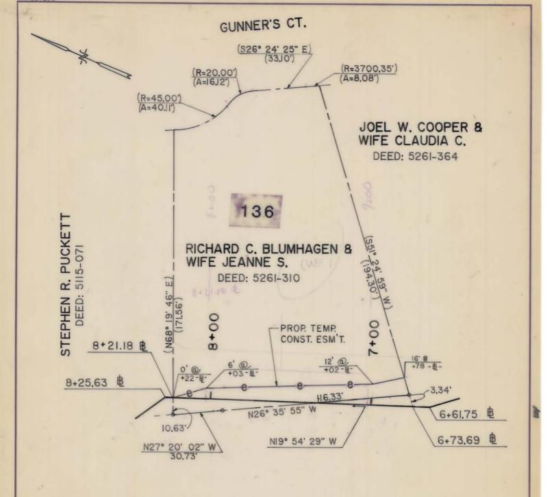
NOTE: Property corners shown circled were located by actual survey. Bearings are based on
