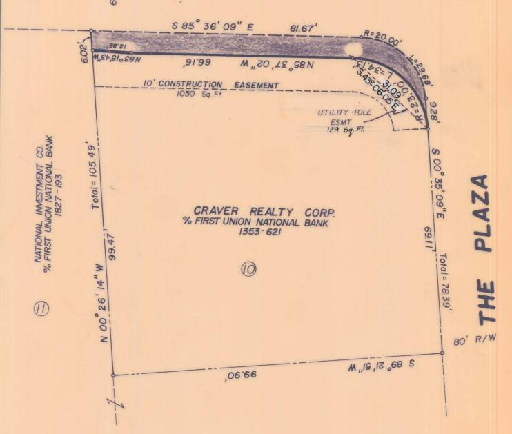
NOTE: PROPERTY CORNERS NOTED WERE LOCATED BY ACTUAL SURVEY BEARINGS ARE BASED ON DEED BOOK 2747 PAGE 477. THIS MAP WAS PREPARED FOR THE PURPOSE OF RIGHT OF WAY OR EASEMENT ACQUISIT-ION ONLY, AND IS NOT INTENDED TO BE A BOUNDARY SURVEY OF THE PROPERTY SHOWN
