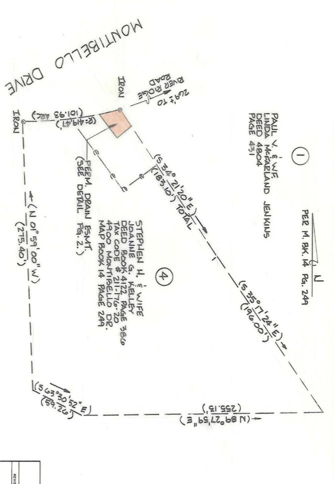
PERM. DRAINAGE ESM'T ACQUIRED: 509 SQ. FT. = 0.0117 AC. TOTAL AREA (BY DEED): 46,435 SQ. FT. = 1.066 AC.
