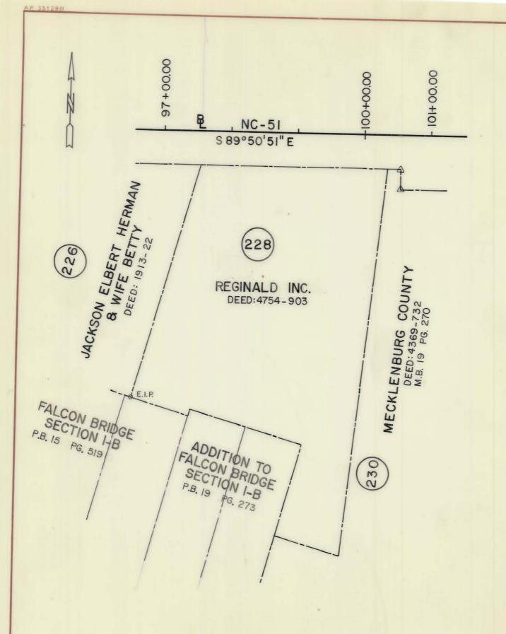
NOTE: Property corners shown circled were located by actual survey. Bearings and distances shown in parenthesis are based on deed information. Bearings are based on
