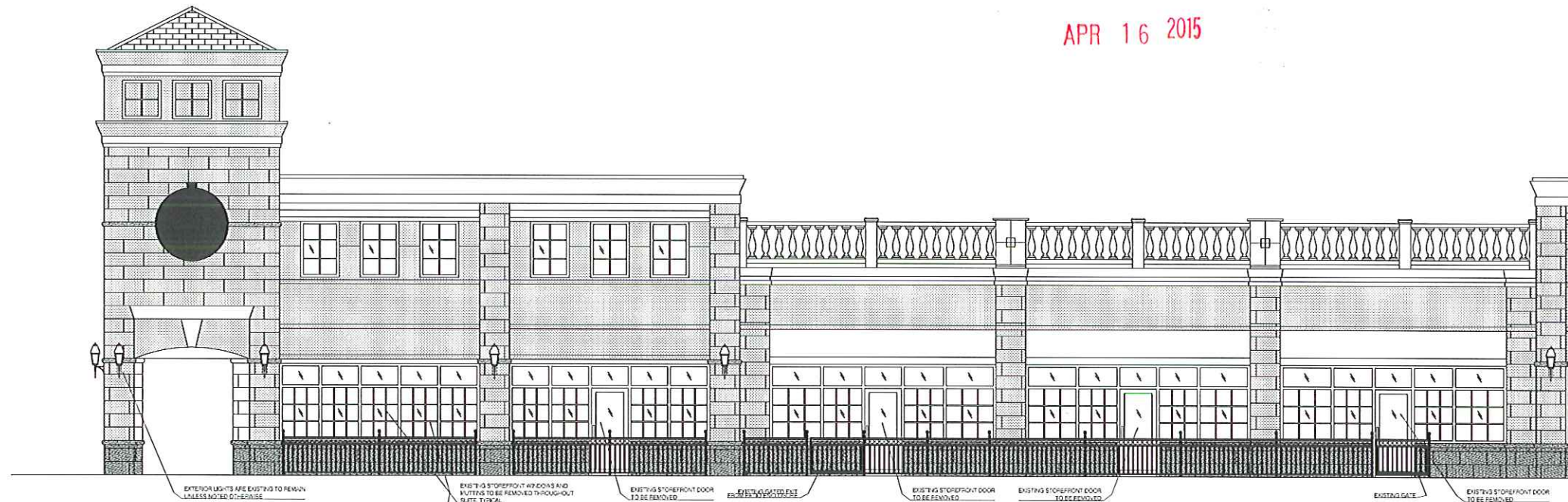
2 NORTH ELEVATION FACING PATIO SCALE: 1/4"=1'-0"
