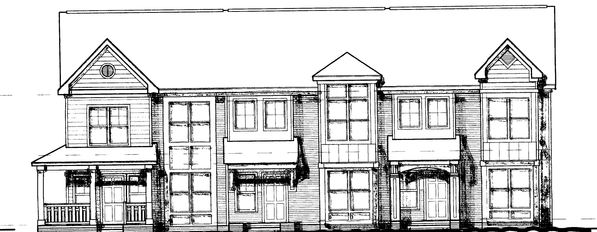
5 FRONT ELEVATION - REAR LOAD - THREE UNIT BLDG 1/4" = 1'-0"
