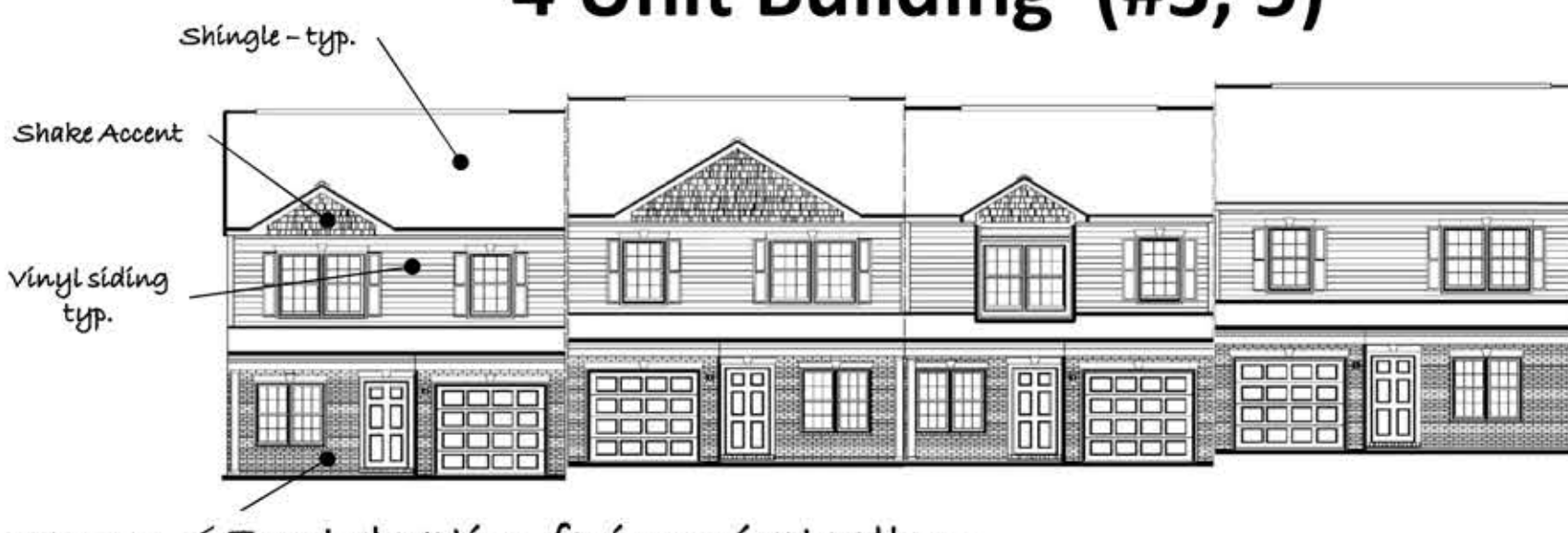
Front elevation facing private alleys 55% Brick
