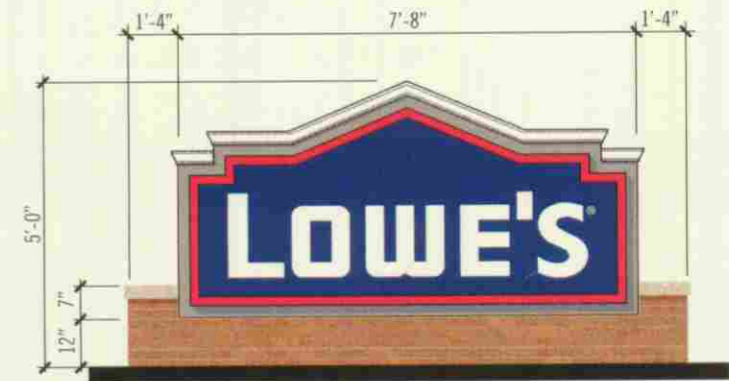
MONUMENT SIGN Double face, Internally lit (PS-4) Area of sign face = 31.66 sf
