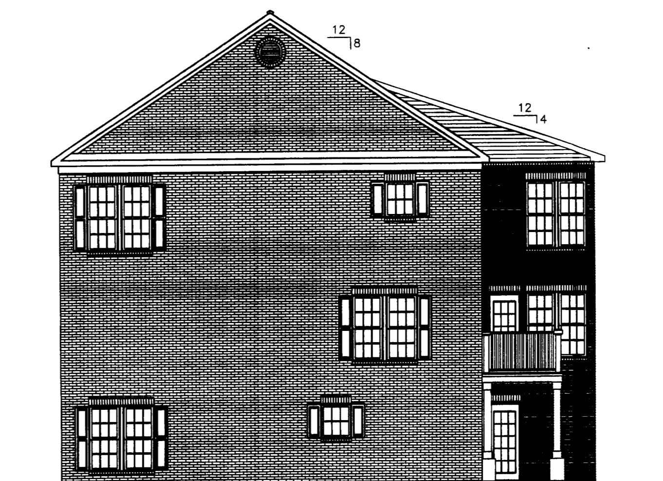
13 FRONT LOADED SIDE ELEVATION @ CHURCH / WINNIFRED A-6 SCALE: 1/8" = 1'-0" (WITH OPTIONAL THREE-STORY SUNROOM) (NOTE: THIS ELEVATION ONLY WHERE THE BUILDING SIDE OF FRONT LOADED UNITS ABUT CHURCH OR WINNIFRED STREETS)
