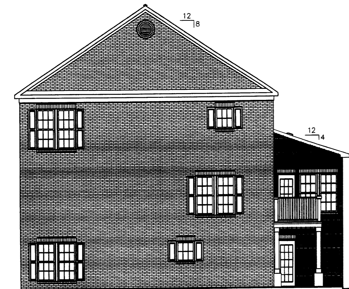
11 FRONT LOADED SIDE ELEVATION @ CHURCH / WINNIFRED A-6 SCALE: 1/8" = 1'-0" (WITH OPTIONAL TWO-STORY SUNROOM) (NOTE: THIS ELEVATION ONLY WHERE THE BUILDING SIDE OF FRONT LOADED UNITS ABUT CHURCH OR WINNIFRED STREETS)
