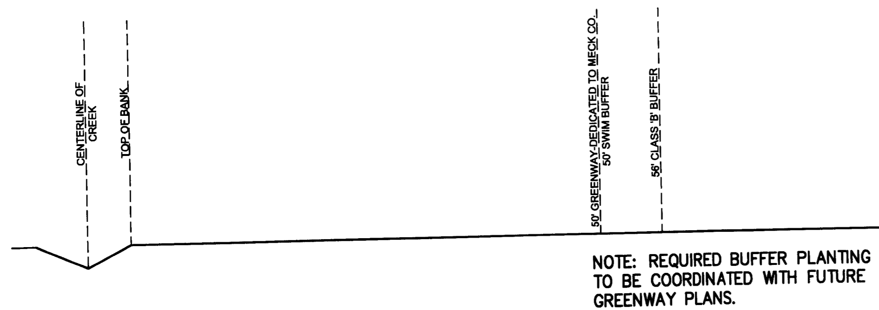
3 CREEK CROSS SECTION A - 35' SWIM BUFFER 1/8"=1'-0" RZ-4
