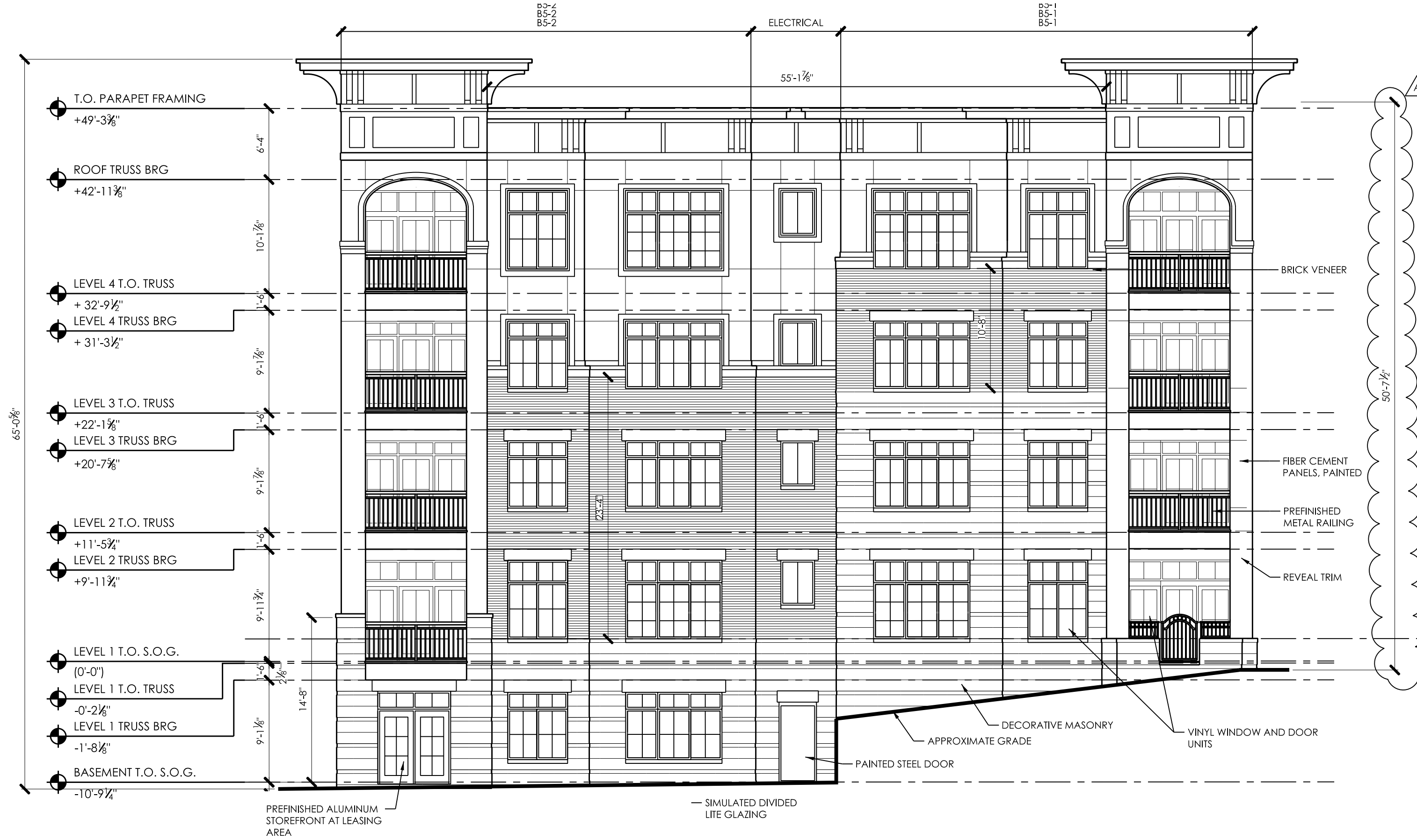
2 EAST ELEVATION AT LEASING / STEP 1/8" = 1'-0"
