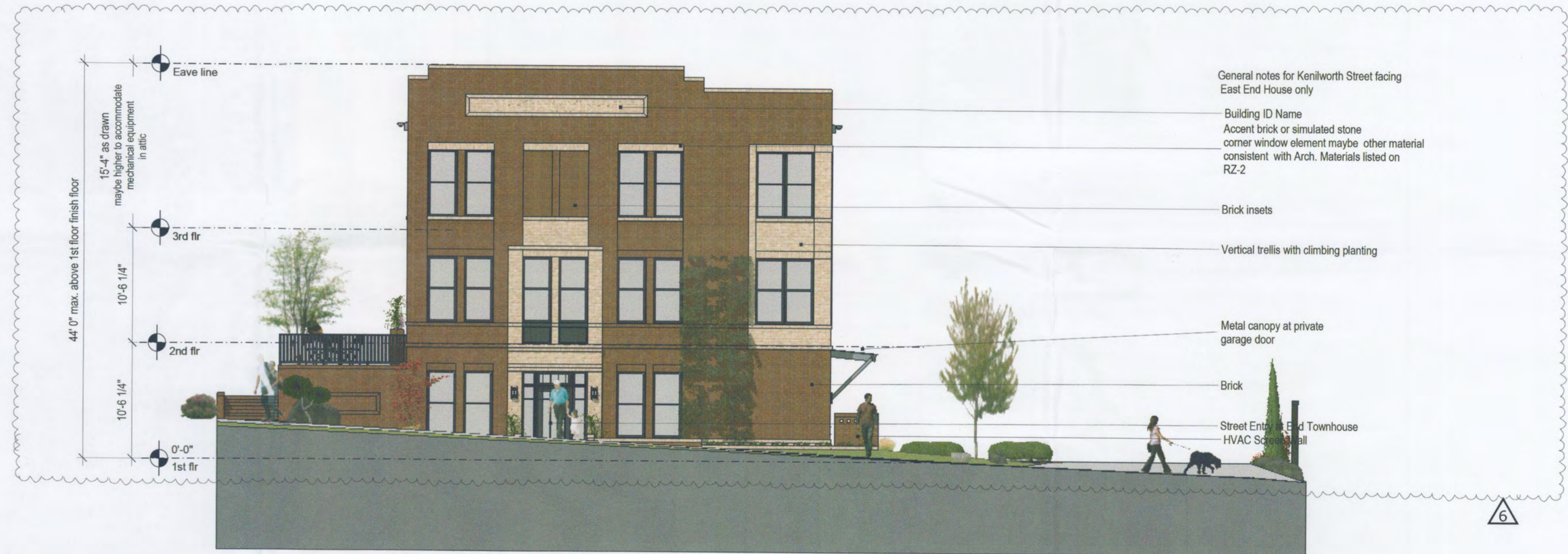
C :: East Elevation (Kenilworth Avenue) RZ3 scale: 1/8"=1' 0"
