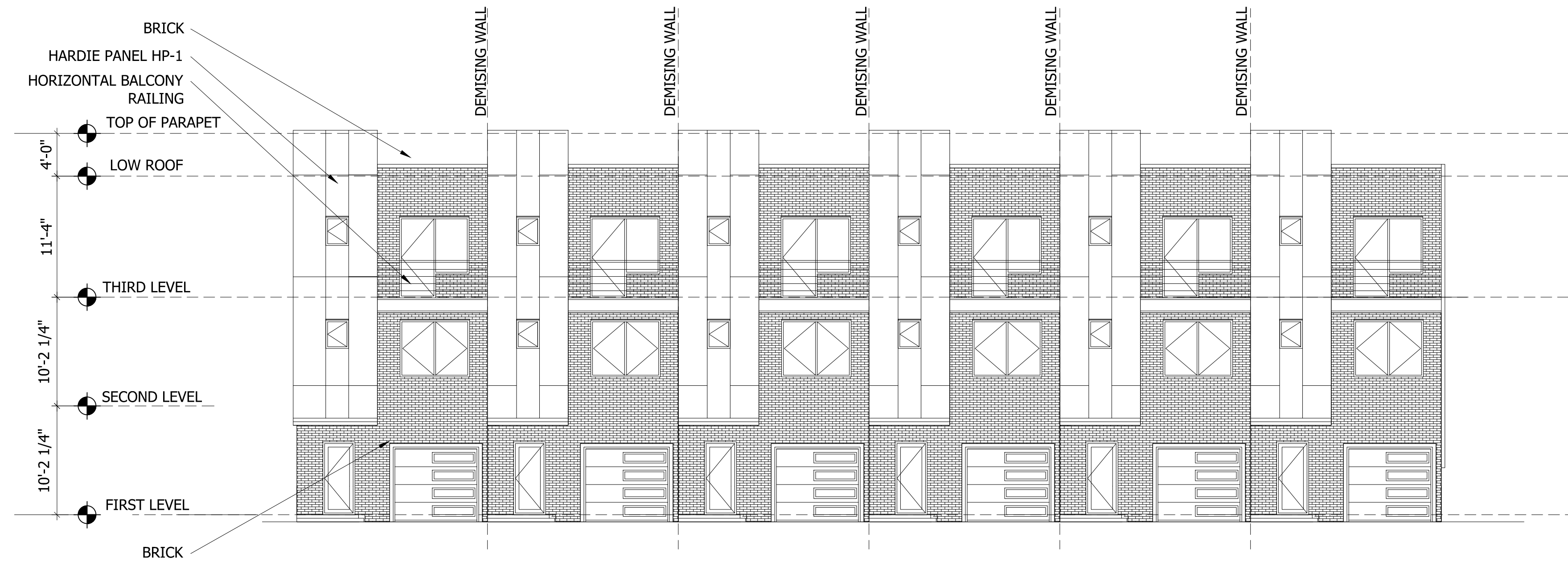
1 ALLEY / GARAGE SIDE ELEVATION RZ3.0 SCALE: 1/8" = 1'-0"
