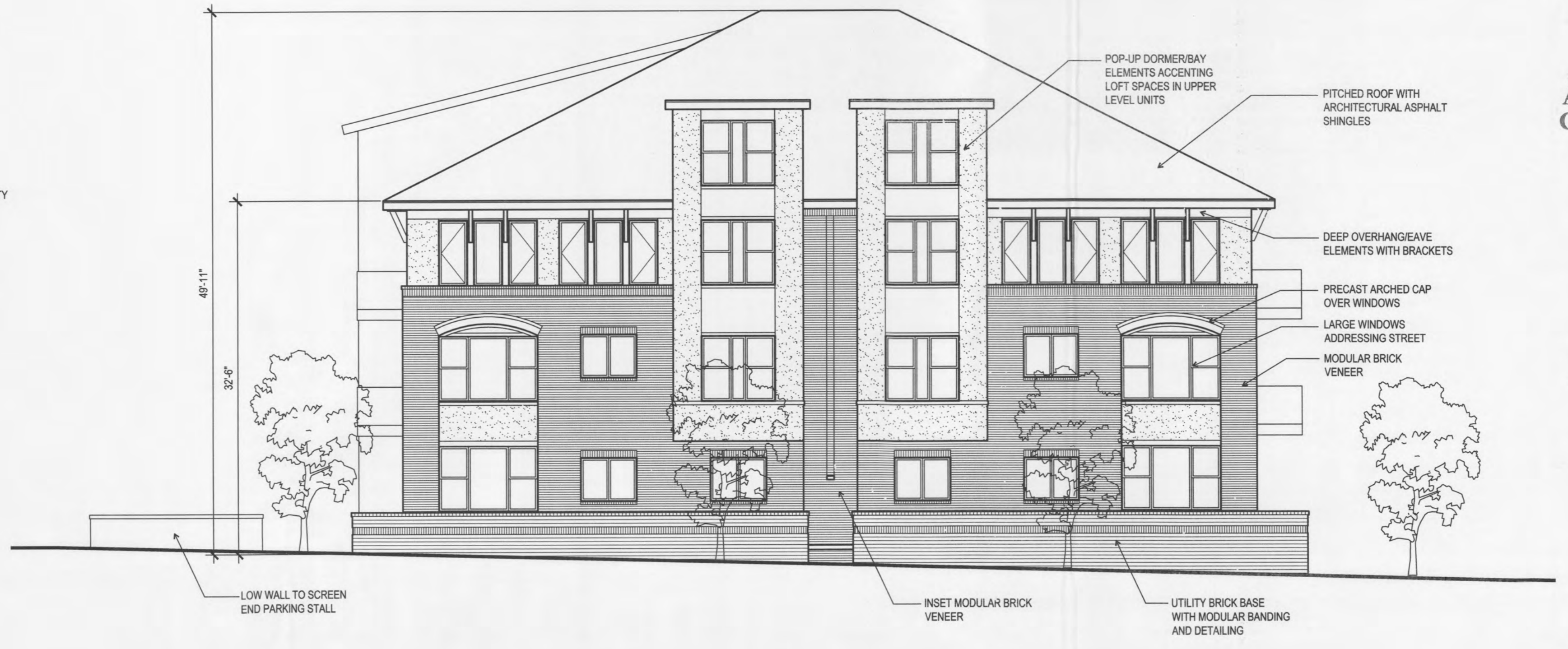
2 BUILDING 2 STREET ELEVATION RZ.03 1/8" = 1'-0"
