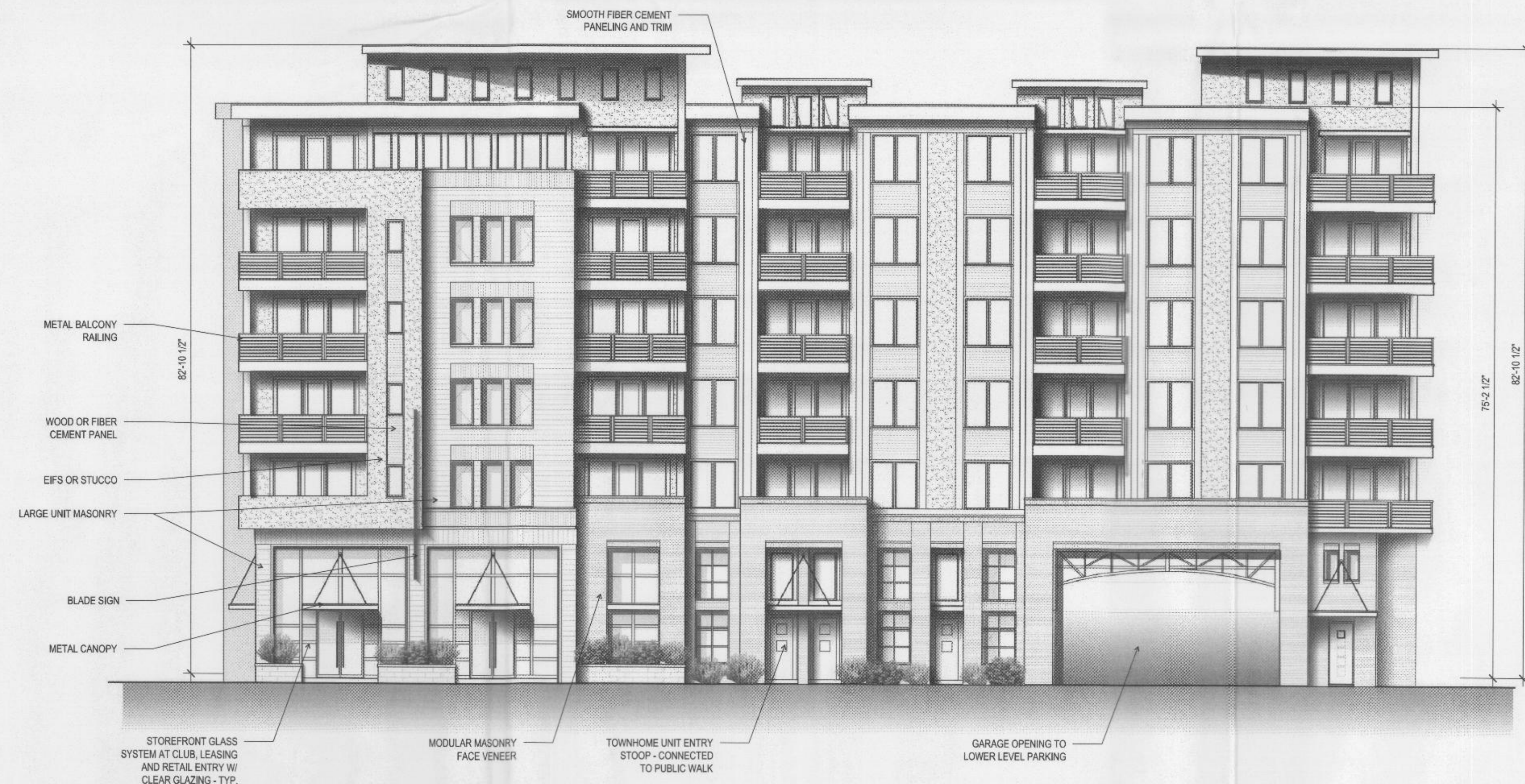
1 SOUTH BLVD ELEVATION A.L.D. 3/32" = 1'-0"
