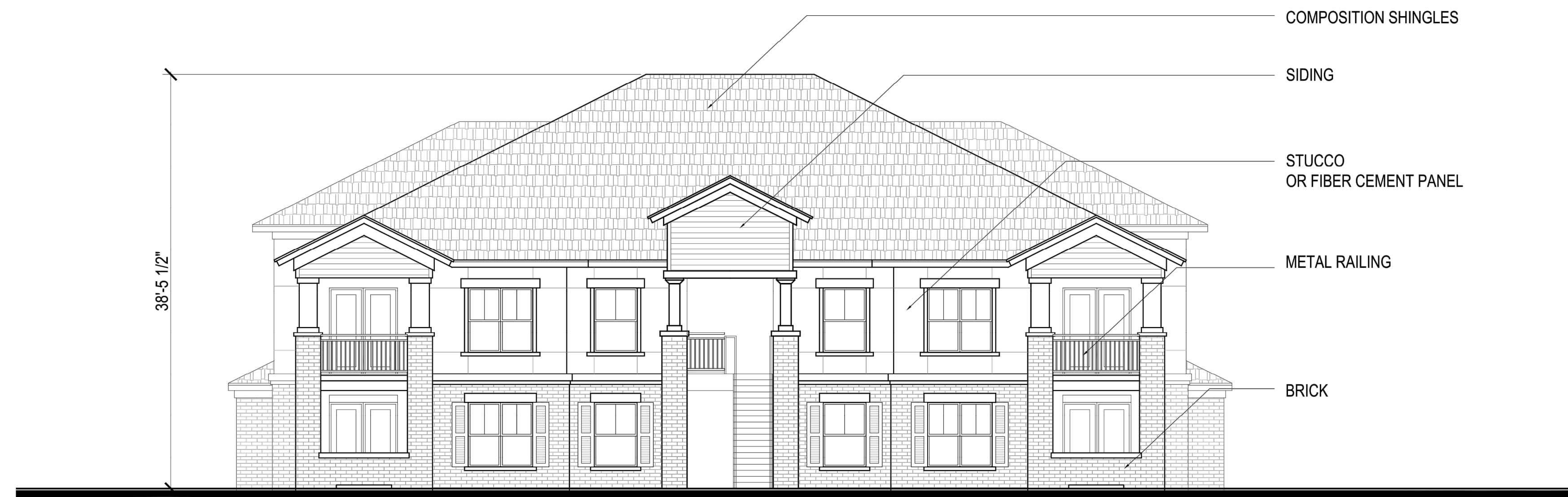
BUILDING TYPE II - FRONT/REAR ELEVATION
