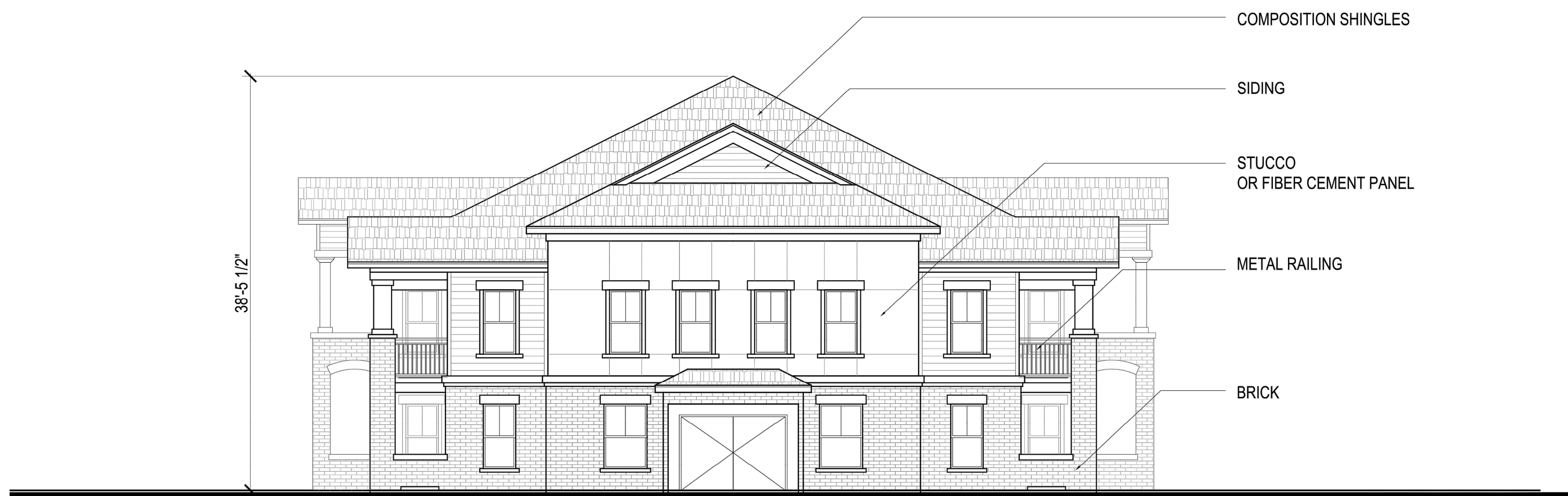
BUILDING TYPE II - RIGHT/LEFT ELEVATION
