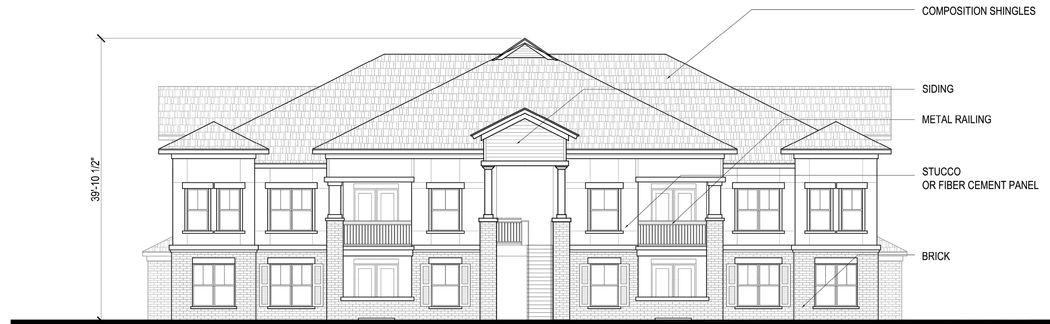
BUILDING TYPE I - FRONT/REAR ELEVATION
