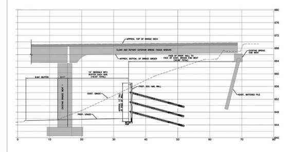
Soil design parameters have been developed from the laboratory test program and empirical relationships between soil types and N-values. These design parameters are presented in the generalized soil profile, Figure 4, in Appendix A and have been utilized in the evaluation of the soil nail wall.
